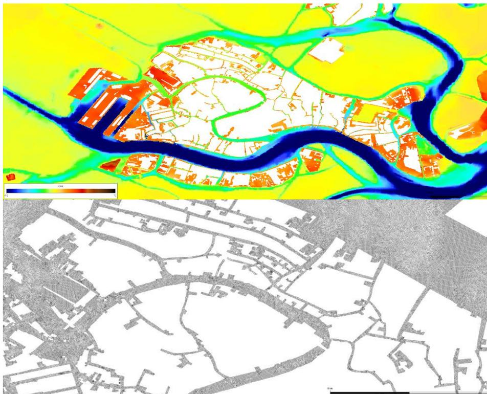
Figure 4. Zoom in the Venice lagoon (Northern Italy) used to illustrate the features of the new topobathymetry (top panel) and mesh (bottom panel) accounting for inundation and building impact on the storm surges.
