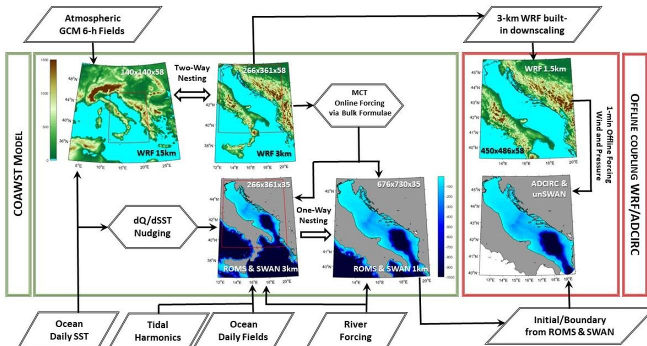
Figure 1. Modules of the AdriSC modelling suite. The basic module is based on the COAWST Model (green frame) and is run for 31-year long periods. The storm surges are run with the nearshore module consisting in the Offline Coupling WRF/ADCIRC (red frame) for a period of 2 days.
