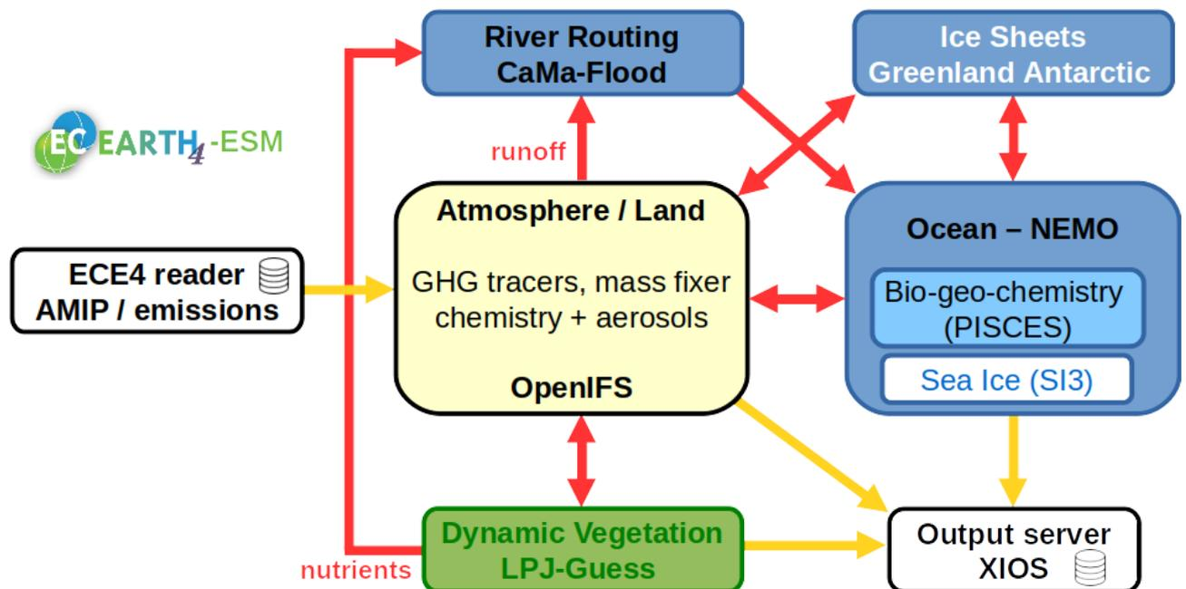
**Figure 1:** A schematic representation of the components and their coupling in the full EC-Earth4 ESM version ECE4-ESM
