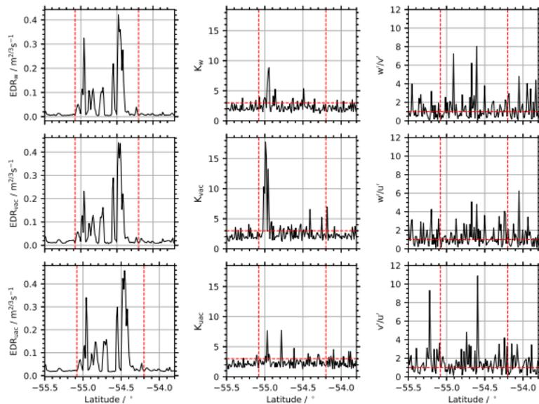
**Figure 1:** Energy dissipation rate (left column), kurtosis (middle column), and anisotropy measure (right column) as function of latitude for the three velocity components in aircraft-related coordinate system  $w$ ,  $vac$ ,  $uac$  from top to bottom, respectively. Red vertical lines frame the entire turbulence segment.
