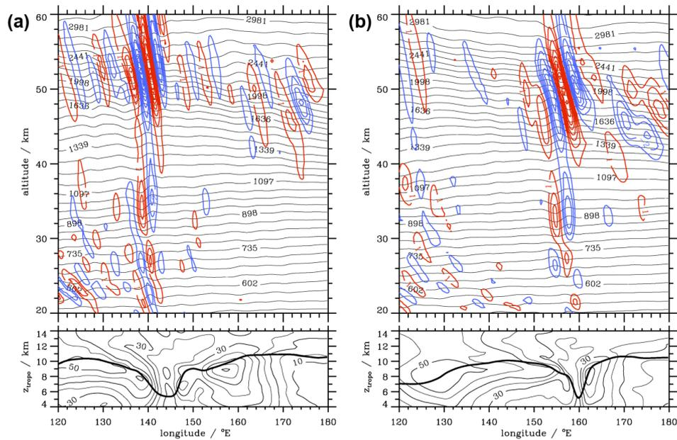
**Figure 5:** Temperature perturbations  $T'_{ERA5}$  (K, red and blue contour lines) and potential temperature (K, black lines in logarithmic scaling) along 55°S on 17 July 2014 15 UTC (a) and 18 July 2014 09 UTC (b). The bottom panels depict the height of the dynamical tropopause (thick black lines, meridional average from 52.5°S to 57.5°S) and the horizontal wind (m s<sup>-1</sup>, thin black lines) at the same instances. Data: One hourly ERA5 data.
