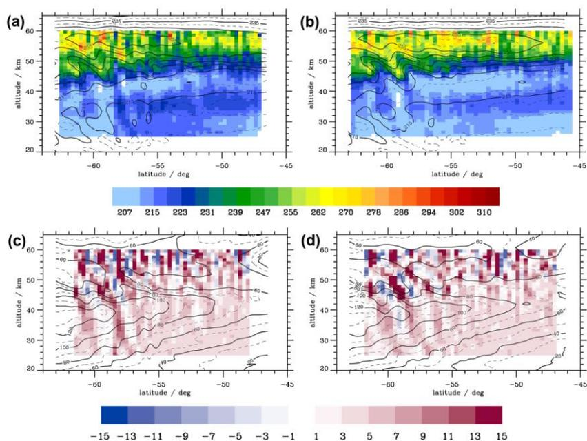
**Figure 4:** (a, b) GV Rayleigh lidar temperature (K, color coded) and IFS temperature (K, black contour lines) and (c, d) temperature perturbations  $T'$  from the Rayleigh lidar (K, color coded) and IFS horizontal wind ( $\text{m s}^{-1}$ , black contour lines) for the outbound (a, c) and inbound (b, d) legs of RF25. Data: 180 s mean values of the Rayleigh lidar observations and HRES IFS.
