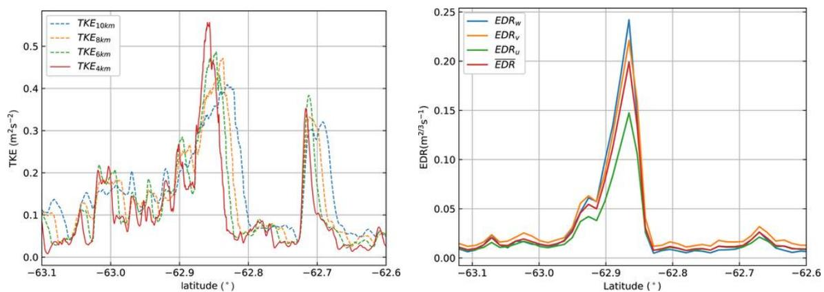
**Figure 2:** Left; Specific turbulent kinetic energy derived from different subleg lengths as indicated by the different colors and line styles, along HALO's flight path through the CAT encounter. Right: Cubic root of the energy dissipation rate ( $EDR = \varepsilon^{1/3}$ ) for all wind components in an aircraft-related coordinate system and the geometric mean  $\overline{EDR}$  calculated from all wind components, along the same flight path.
