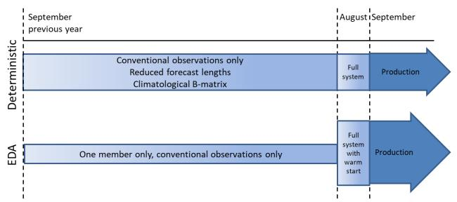
Figure 1: Schematic setup for the spin-up periods to reduce SBU costs.
