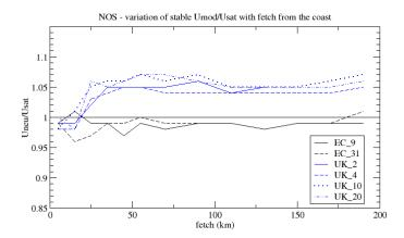
Figure 8 – ECMWF and UKMO results for wind blowing off the coast of East Anglia. All the available resolutions are shown.
