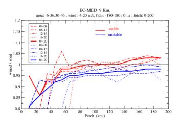
Figure 1 – Ratio model/scatterometer wind speeds as a function of "fetch". The blue limes refer to unstable conditions, the red ones to stable ones
