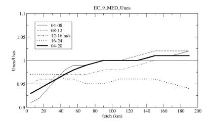
Figure 6 – Ratio between model neutral and scatterometer wind speed values as a function of fetch (km) and of the wind speed at the measurement point. The dark line is the average of all the data.
