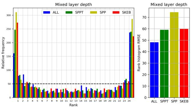
Figure 2. Rank histogram and associated root mean square difference compared to the flat p.d.f., for mixed layer depth data from stochastic physics experiments and glider profile observations. Four experiments are compared, either with all perturbation schemes applied simultaneously, or individually.
