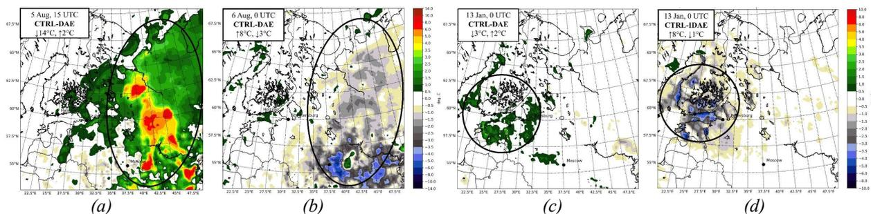
**Figure 3:** Difference fields for the air temperature at 2 m between the control/reference vs. modified runs (a,c) CTRL-DAE and (b,d) CTRL-IDAE for selected dates in (a,b) August and (c,d) January 2010.
