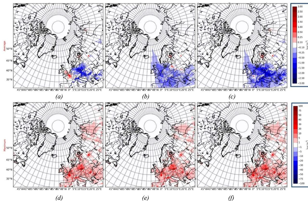
**Figure 8:** Difference fields between CTRL&DAE (a,d), CTRL&IDAE (b,e), CTRL&DAE+IDEA (c,f) runs with the Enviro-HIRLAM model for January's monthly averaged (a,b,c) and maximum (d,e,f) concentration of black carbon.
