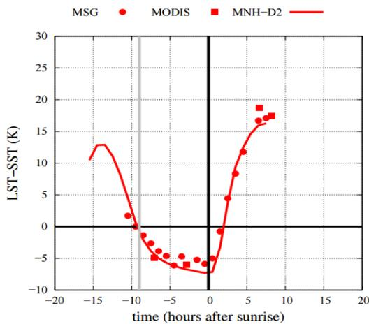
Figure 6. Modelled and satellite derived surface temperature differences between land and sea for IOP 3. The temperatures are averaged over a similar area covering: the center of the Campos basin (LST) and the bay over the sea in front of the Campos basin (SST). Time is shifted to the sunrise hour (black vertical line) and sunset is indicated with a grey line.
