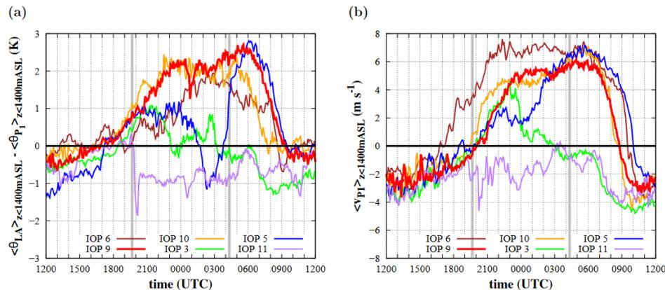
Figure 18. (a) Time series of the difference of the vertically-averaged (from the ground up to 1400 m ASL) potential temperature between Lannemezan (LA) and the exit of the Aure Valley. (b) The same as (a) but for the averaged v-component of the wind at the exit of the valley. The vertical grey lines indicate sunset and sunrise instants and the black horizontal one shows the position where the wind or the temperature difference are zero.
