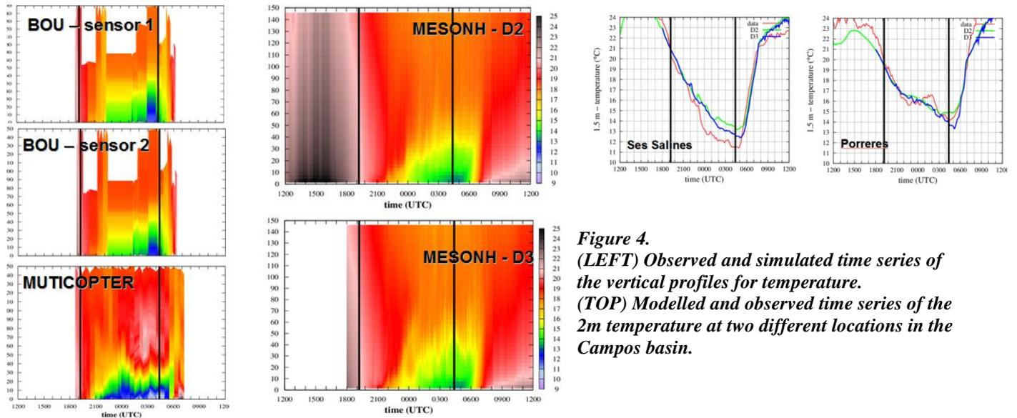
Figure 4. (LEFT) Observed and simulated time series of the vertical profiles for temperature. (TOP) Modelled and observed time series of the 2m temperature at two different locations in the Campos basin.
