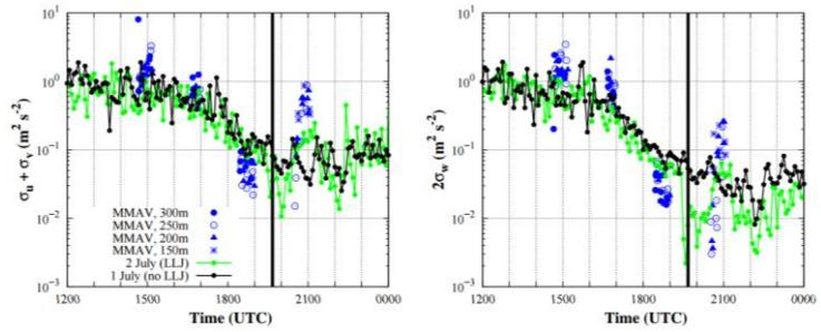
**Figure 18b.** The same as a but for the (LEFT) horizontal  $\sigma_u + \sigma_v$  and (RIGHT) vertical  $2\sigma_w$  variances computed from the tower observations at 60 m AGL during IOP 9 (without an LLJ, black line) and IOP 10 (with an LLJ, green line), together with those derived from  $M^2AV$
