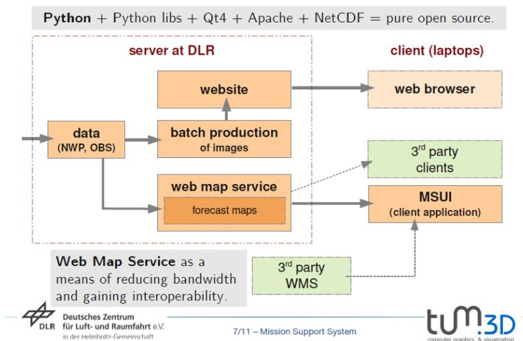
**Fig. 1:** Conceptual design of the Mission Support System developed in collaboration between the DLR and the Technical University of Munich.
