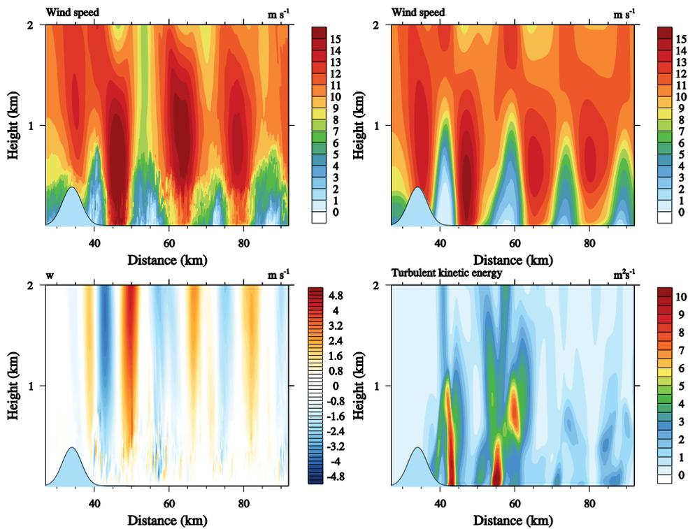
**Figure 1:** Vertical cross-sections ( $x$ - $z$ ) of the flow field at the middle of the computational domain in the  $y$  direction. From top left: instantaneous  $u$  wind component at  $t = 6$  h; mean  $u$  wind component between  $t = 5.5$  h and  $t = 6$  h; instantaneous  $w$  wind component at  $t = 6$  h; explicitly resolved turbulent kinetic energy between  $t = 5.5$  h and  $t = 6$  h.
