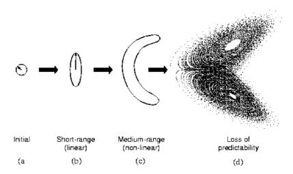
**Figure 1.1** A schematic illustration of the growth of an isopleth of the forecast error probability distribution function, from (a) initial phase, to (b) linear growth phase, to (c) nonlinear growth phase, to (d) loss of predictability. See text for further details.
