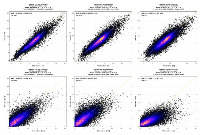
Figure 4. Forecast verification for 2-m temperature (top) and 10-m wind speed (bottom) for the month of June 2021. hm750m (left), harmonie (centre) and HRES (right).
