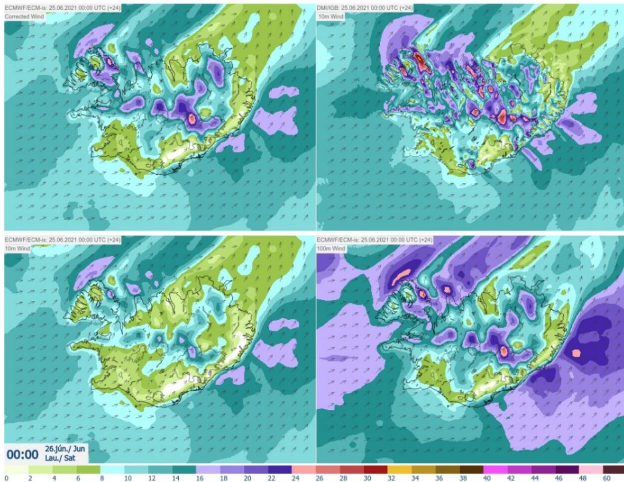
Figure 1. A comparison of 10-m wind speed. HRES post-processed (top left), HARMONIE-AROME IGB DMO (top right), HRES 10-m DMO (bottom left) and HRES 100-m DMO (bottom right). 24-hour forecasts valid on 26 June 2021 00 UTC.
