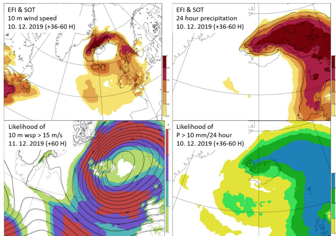
Figure 6. EFI & SOT of 10-m wind speed and 24-hour accumulated precipitation as well as the likelihood of wind speed exceeding 15 m/s and precipitation 10 mm/24 hours in the weather event of 10-12 December 2019.
