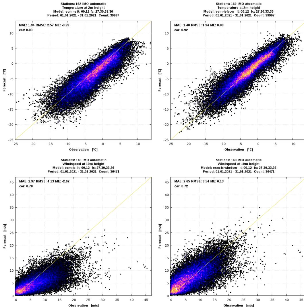
Figure 5. Scatterplots of observed and forecasted 2-m temperature (top) and 10-m wind speed (bottom). Left: HRES DMO. Right: HRES post-processed. Forecast length 27-36 hours and forecast period January 2021.
