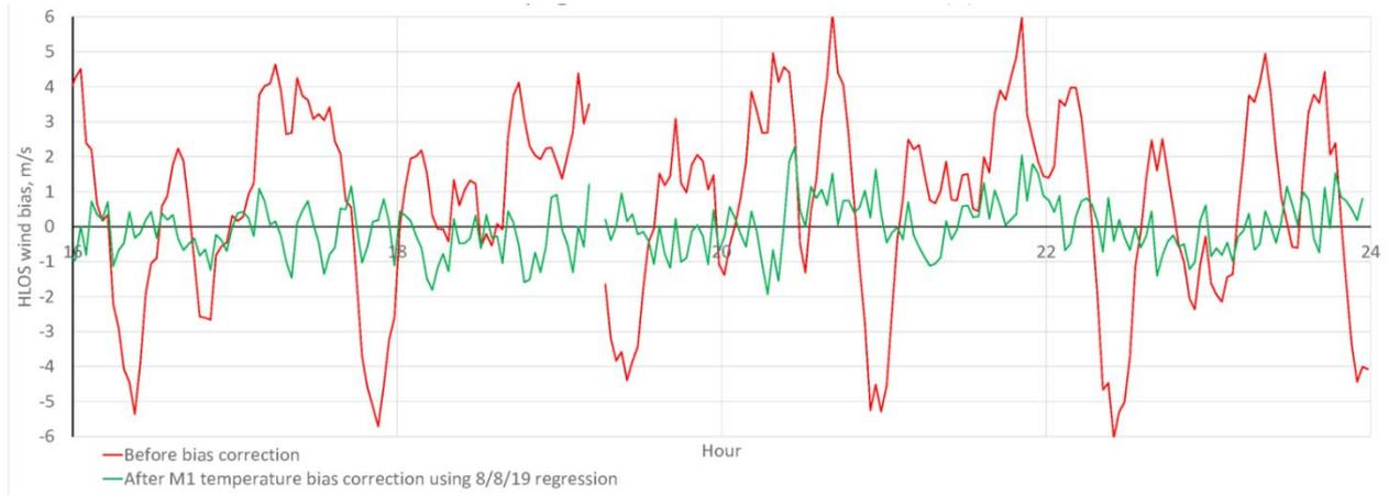
Figure 23. L2B Rayleigh-clear HLOS wind bias versus time (between 16:00 and 23:59 UTC) on 9 August 2019, in 2-minute samples of mean(O-B) for all wind observations. The red line is before any bias correction and green is after an M1 bias correction using the linear regression coefficients calculated from the previous day (8 August 2019), as shown in Figure 22.
