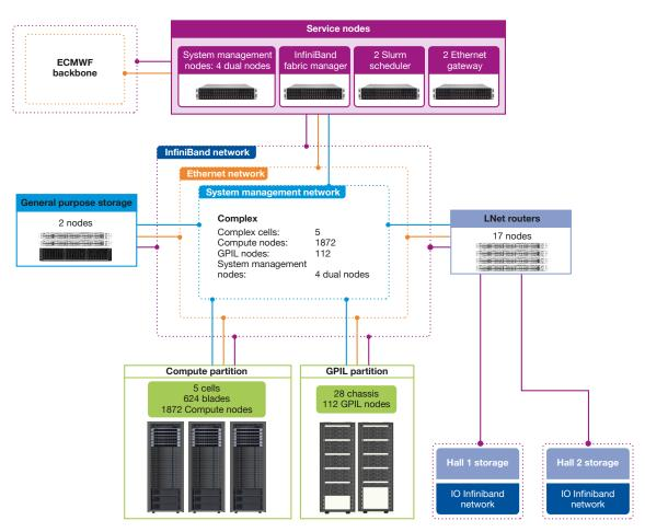
Figure 3 Overview of an HPC cluster. There are four of these in the system.
