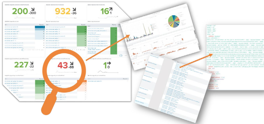
Figure 3 A customised dashboard to monitor and troubleshoot Web-API service activity in near real time. A suspicious spike in ‘failing’ requests can be investigated further by drilling down, through several bespoke dashboards and tools, to the root of the problem and viewing associated events.
