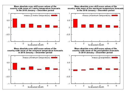
Fig.7 Mean Absolute Error Skill Score of ensemble means of 2 m, maximum and minimum temperature and precipitation for the 6 forecasted months in a forecast for 2018. Reference forecast was the 30-year climatological mean.
