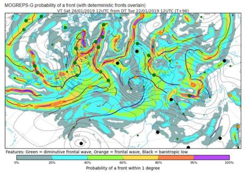
Fig.1 An example of the objective fronts probability maps in MOGREPS-G. Fronts from the deterministic model (represented by blue and red lines) can be seen to be an outlier compared to the ensemble consensus (coloured areas) over both the Atlantic Ocean and Northwest Europe.
