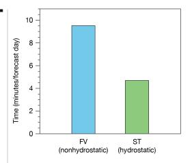
For added flexibility, it is also developing a new, nonhydrostatic dynamical core which uses the finite-volume method. In 2018, this 'Finite-Volume Module' (FVM) was shown to perform well compared to the current dynamical core in benchmark tests, and its computational cost was reduced substantially. Tests have shown that it holds great promise in terms of computational efficiency for global nonhydrostatic forecasts at high resolution run on future exascale high-performance computing facilities.
