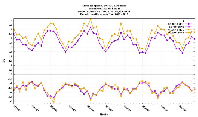
Fig. 5 Monthly values of RMSE and bias for forecasted 10-metre wind speed (m/s) for the time period 2013—2017. Forecast length of 48 hours (purple) and 120 hours (yellow), initialized at 00 UTC and 12 UTC.
