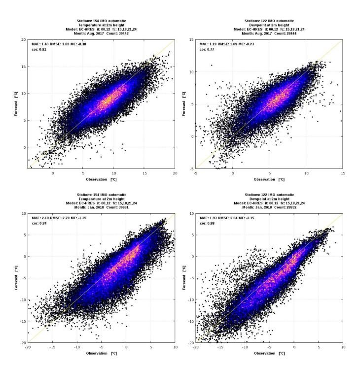
Fig. 3 Scatter plots of 2-metre temperature (°C, left) and dew point (°C, right) forecasts and observations for August 2017 (top) and January 2018 (bottom). ECMWF HRES forecast length 15, 18, 21 and 24 hours, initialized at 00 UTC and 12 UTC.
