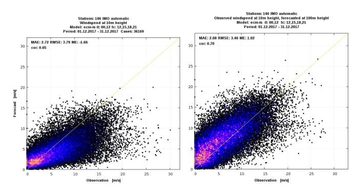
Fig. 4 Scatter plots of 10-metre wind speed (m/s, left) and 100-metre wind speed (m/s, right) forecasts and observed wind speed at 10 metre for December 2017. ECMWF HRES forecast length 12,15, 18, and 21, initialized at 00 UTC and 12 UTC.
