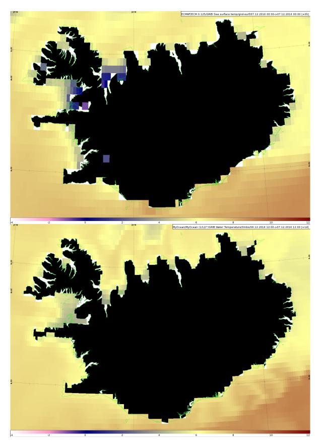
Fig. 6 Sea surface temperature (°C) around Iceland in ECMWF analysis on 7 December 2016 00 UTC (top) and MyOcean 24 hour forecast valid 7 December 2016 12 UTC. The sub-zero SSTs in the fjords in west and northwest Iceland in the ECMWF analysis are incorrect.
