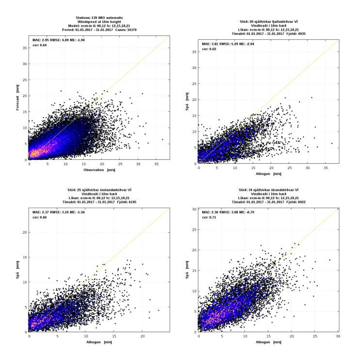
Fig. 3 Scatter plot of 10-metre wind speed (m/s) forecasts and observations for forecasts length 12, 15, 18 and 21 hours, initialized at 00 UTC and 12 UTC for all stations (top left), highland stations only (top right), inland stations only (bottom left) and coastal stations only (bottom right). January 2017 HRES.
