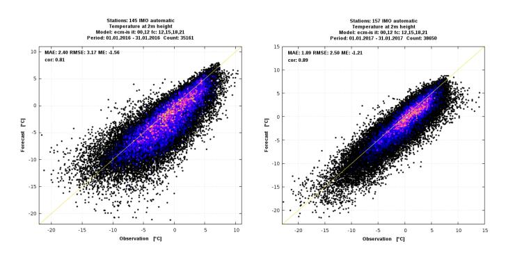
Fig. 2 Scatter plot of 2-metre temperature (°C) forecasts and observations for forecasts length 12, 15, 18 and 21 hours, initialized at 00 UTC and 12 UTC for January 2016 (left) and 2017 (right). ECMWF HRES.
