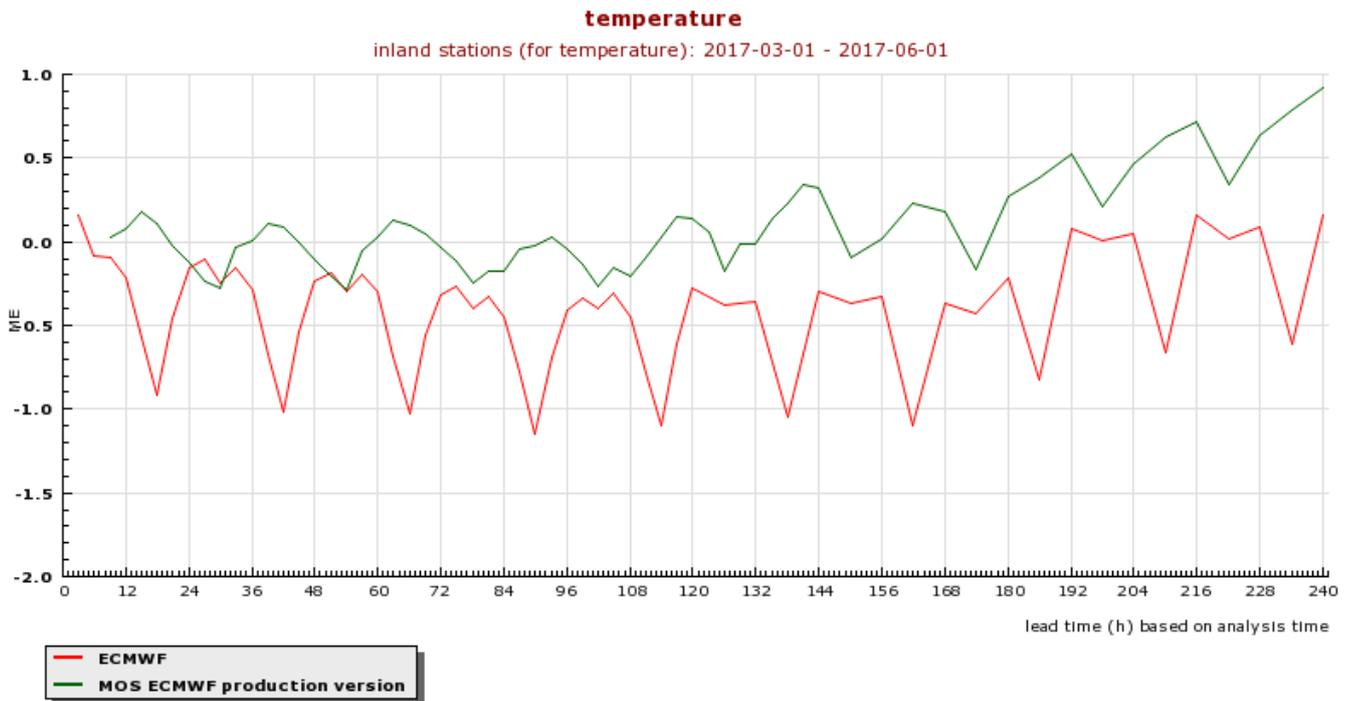
Fig 3. Mean error of 2m temperature of 00utc analysis times of spring as a function of forecast length for ECMWF (red line) and MOS calibrated ECMWF (green line) shows how MOS is able to correct the cold evening bias.
