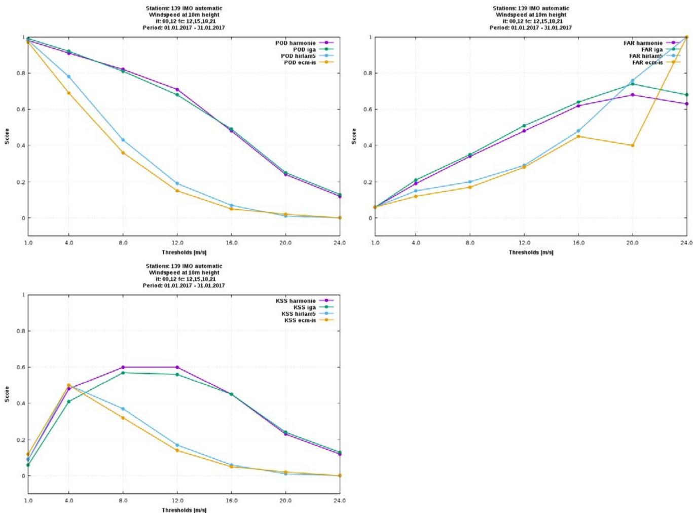
Fig. 5 Skill scores for 10-metre wind speed from HARMONIE-AROME (purple), IGA (green), HIRLAM5 (blue) and HRES (yellow) for January 2017. Top left: POD, top right: FAR and bottom: KSS.
