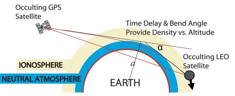
We assimilate bending angle as a function of impact parameter (~height).
