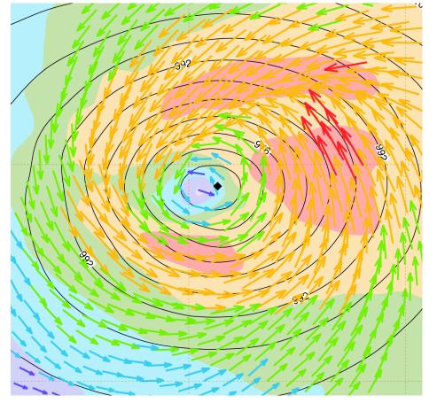
But if the model has a error in the cyclone position sometimes the **wrong ASCAT wind is selected** (below is a <u>bad</u> example, TC *PAM*)
