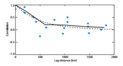
Fig. 3. Distance correlogram of the observation (model+measurement) error  $\hat{\mathbf{R}}^{\text{prior}}$  estimated from Eq. (1), using pairs of distant sites for a same time. The value represented by each blue diamond includes all the common years of one site pair. The thick black line represents the overall median using 400-km bins, and the dotted line an exponential decay with an e-folding length of 500 km.
