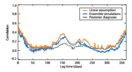
Fig. 2. All-site median of the autocorrelation of the observation error (i.e., model error + measurement error)  $\mathbf{R}$ , estimated at each site with three methods: prior diagnostics with the linear assumption (orange,  $\hat{\mathbf{R}}^{\text{prior}}$  from Eq. 1), prior diagnostics with ensemble simulations (blue,  $\hat{\mathbf{R}}^{\text{prior}}$  from Eq. 1), and posterior diagnostics (grey,  $\hat{\mathbf{R}}^{\text{post}}$  from Eq. 3).
