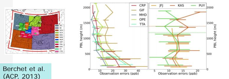
**Fig. 3.** Statistics of the errors projected along ECMWF-simulated PBL height for ML method: median and inter-quartile gap per 250m-high layer. (Left) sites with strong correlations as calculated in Table 2; not displayed site RGL exhibits the same patterns but with higher errors. (Right) Mountain sites with influence from the PBL less prevailing. Dashed lines refer to the station altitude in the model; JFJ is above the maximum simulated PBL height.
