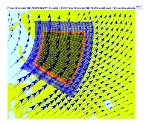
Figure 13: Original semi-Lagrangian transport, showing a wind plot, and greater number of red grid points upwind of MPI task 11
