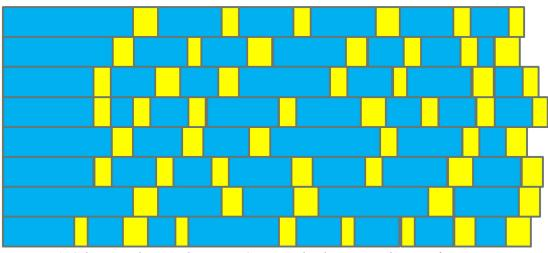
Figure 6: Schematic showing the new IFS approach where Legendre transform computations (blue) are overlapped with associated transpositions (coarray puts-yellow)
