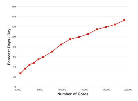
*Figure 16: T3999L137 RAPS13 IFS (CY38R2) hydrostatic forecast model performance on TITAN (Cray XK7)*
