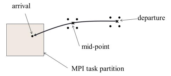
Figure 9: Semi-Lagrangian transport
