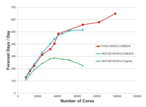
*Figure 15: T2047L137 IFS forecast model performance RAPS12 (CY37R3, on HECToR), RAPS13 (CY38R2, on TITAN)*
