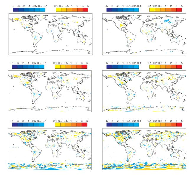
Figure 14: Root Mean Square 2 m temperature forecast error diference between SMOS-DA and CTRL-DA at 24h (top left), 36h (top right), 48h (middle left), 72h (middle right), 96h (bottom left) and 120 (bottom right) forecast lead time. Forecast errors are computed against the own experiment analysis. Values are averaged over the period June to August 2010.
