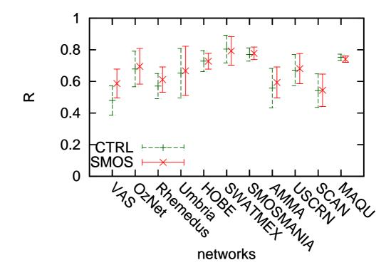
Figure 4: Averaged R value (for the period June-August 2011) between analysis of SMOS-DA and in-situ observations, and between CTRL-DA analysis and in-situ observations, for all networks used in this study. Overlapped are the 95% confidence intervals.
