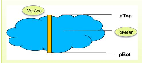
**pMean** – weighed mean of model levels within the cloud, weights proportional to ice (or liquid water) content.
