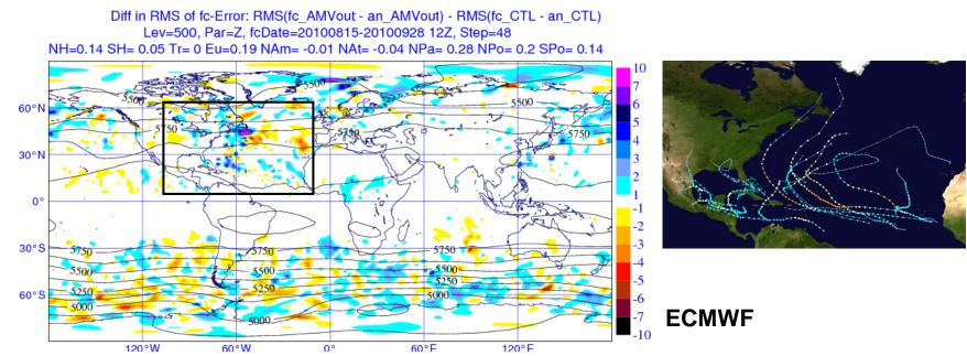
Blue/purple colours represent where the forecast RMS in the reference experiment (containing the AMVs) is smaller than in the denial experiment i.e. positive impact
