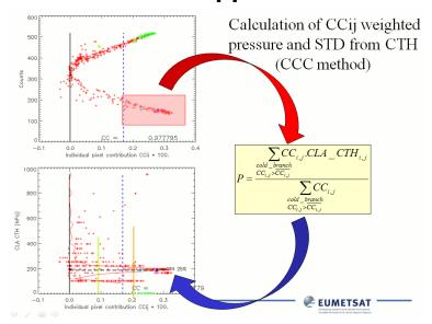
Pixel contribution to the cross correlation coefficient, CCij, is used to select the pixels that contribute most to the tracking
