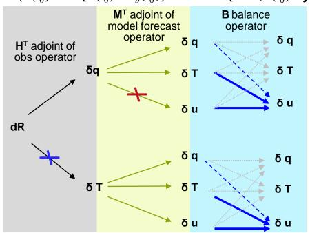
The 4D-Var minimisation process can be regarded as a series of transformations of the observation departure, applying successively the operators:  $\mathbf{R}^{-1}$ ,  $\mathbf{H}^{T}$ ,  $\mathbf{M}^{T}$ ,  $\mathbf{B}$ ;
