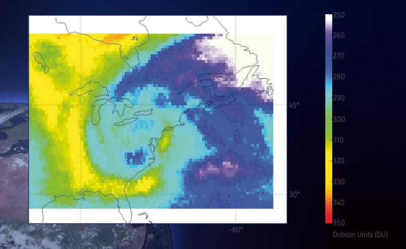
Impact of hurricane Sandy on total ozone, as observed by the GOME-2 instruments of Metop-A and Metop-B, on 30 October 2012. Only the combination of both instruments can map the full region impacted by the storm.
