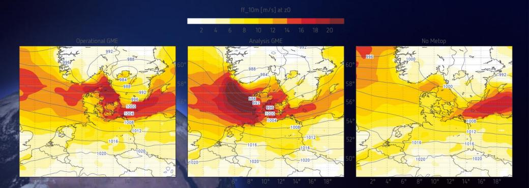
Winter storm "Nicolas": DWD 45-hour forecasts of surface pressure (contour lines) and surface wind speed (shaded areas - units m/s) for 7 February 2011, 21:00 UTC with (left) and without (right) Metop observations, compared to operational analysis (best approximation of ground truth, centre)
