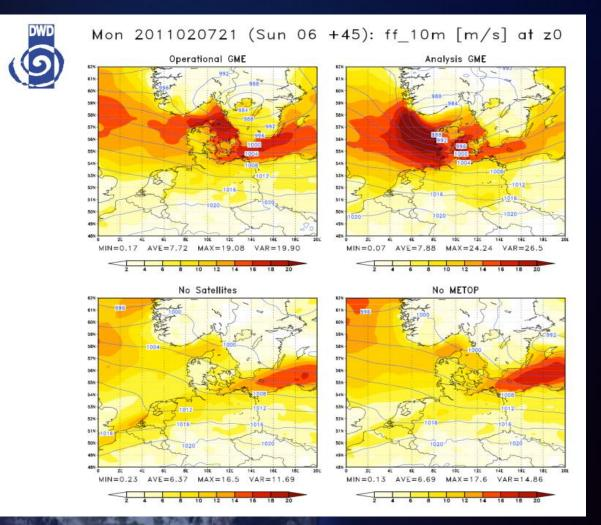
Winter storm "Nicolas": 45 hour forecasts and operational analysis (best approximation of ground truth) of surface pressure (contour lines) and 10m wind speed (shaded areas – units M/S) for 7 February 2011
