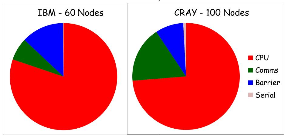
CCE compiler able to vectorise IFS source  $\rightarrow$  Compute relatively faster Aries has fewer hub chips per node than HFI  $\rightarrow$  Comms relatively slower Cray has light-weight kernel on application nodes  $\rightarrow$  Less jitter
