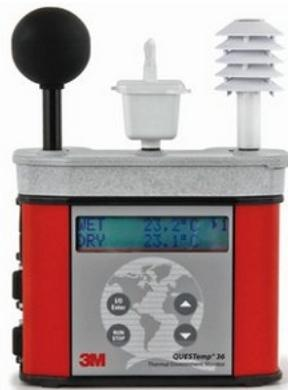
Figure 1 – Three-thermometer device used to estimate the *WBGT* from readings of the ambient air temperature (right), the natural wet-bulb temperature (middle) , and the globe temperature (left). Source: <http://www.heatstress.nl>.
