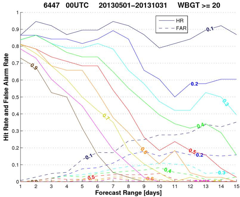
Figure 3 – Hit rate (solid lines) and false-alarm rate (dashed lines) for various probability thresholds (from 0.1, or 10% to 0.9, or 90%). Predicted event: daily maximum *WBGT*  $\geq 20^{\circ}\text{C}$ . 15-day ECMWF ensemble forecasts, all 00-UTC runs. Period: 1<sup>st</sup> May to 31<sup>st</sup> October 2013. Location: Uccle (WMO ID 06447).
