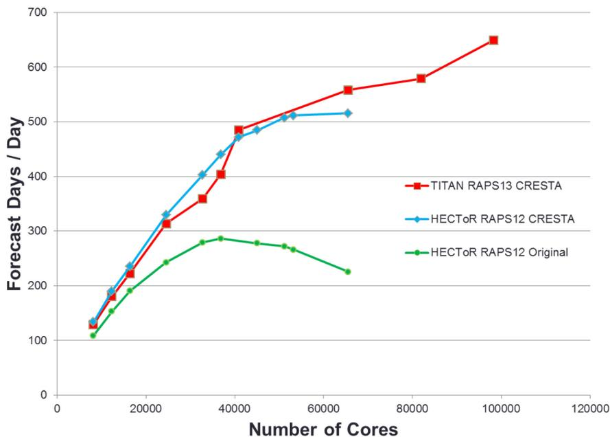
Figure 15: T2047L137 IFS forecast model performance RAPS12 (CY37R3, on HECToR), RAPS13 (CY38R2, on TITAN)
