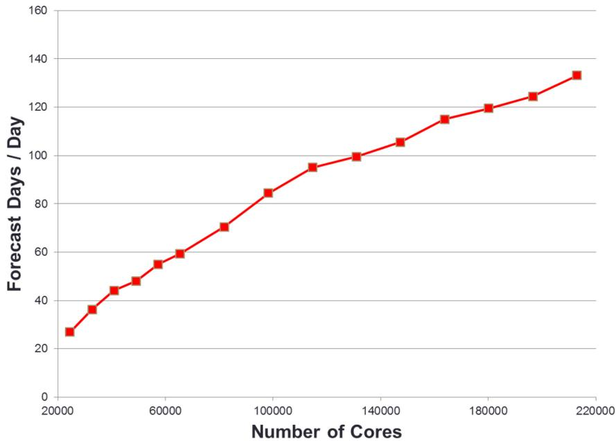
Figure 16: T3999L137 RAPS13 IFS (CY38R2) hydrostatic forecast model performance on TITAN (Cray XK7)
