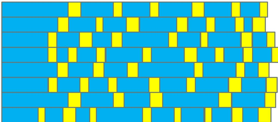
Figure 6: Schematic showing the new IFS approach where Legendre transform computations (blue) are overlapped with associated transpositions (coarray puts-yellow)
