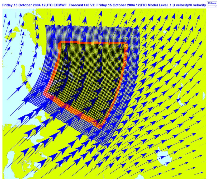
Figure 13: Original semi-Lagrangian transport, showing a wind plot, and greater number of red grid points upwind of MPI task 11
