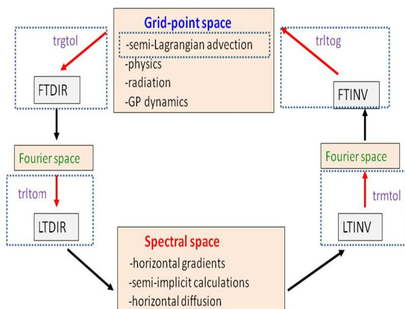
Figure 2: IFS time step: Current areas of IFS optimisation showing where coarray optimisations have been applied (the dotted boxes)
