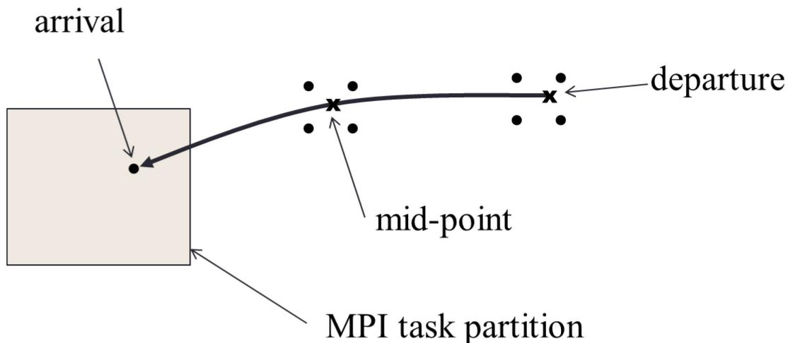
Figure 9: Semi-Lagrangian transport
