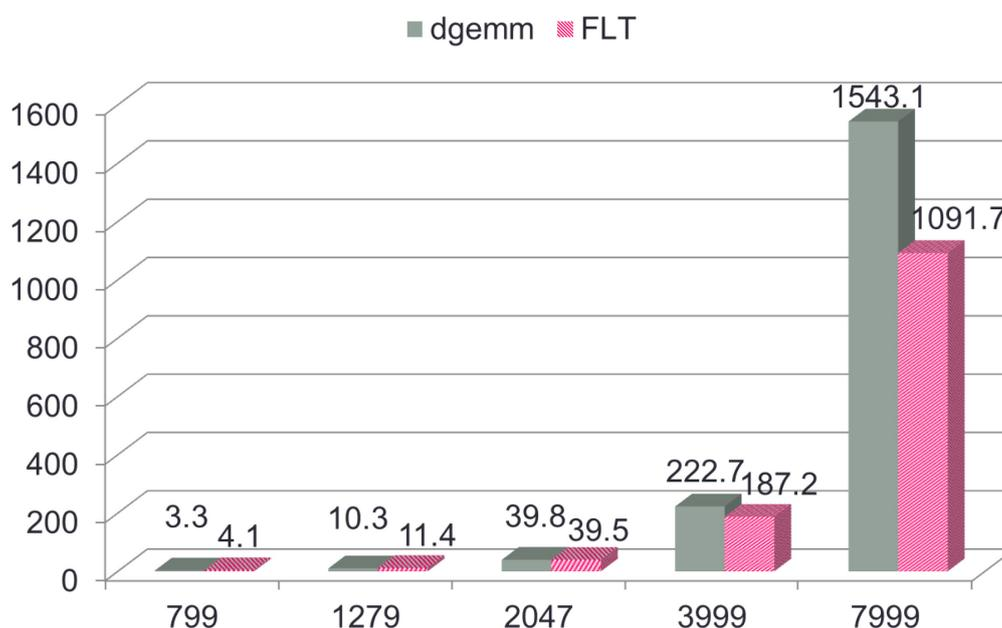
Figure 3: Average wall-clock time compute cost [milli-seconds] per spectral transform, where dgemm represents the old algorithm and FLT the new algorithm
