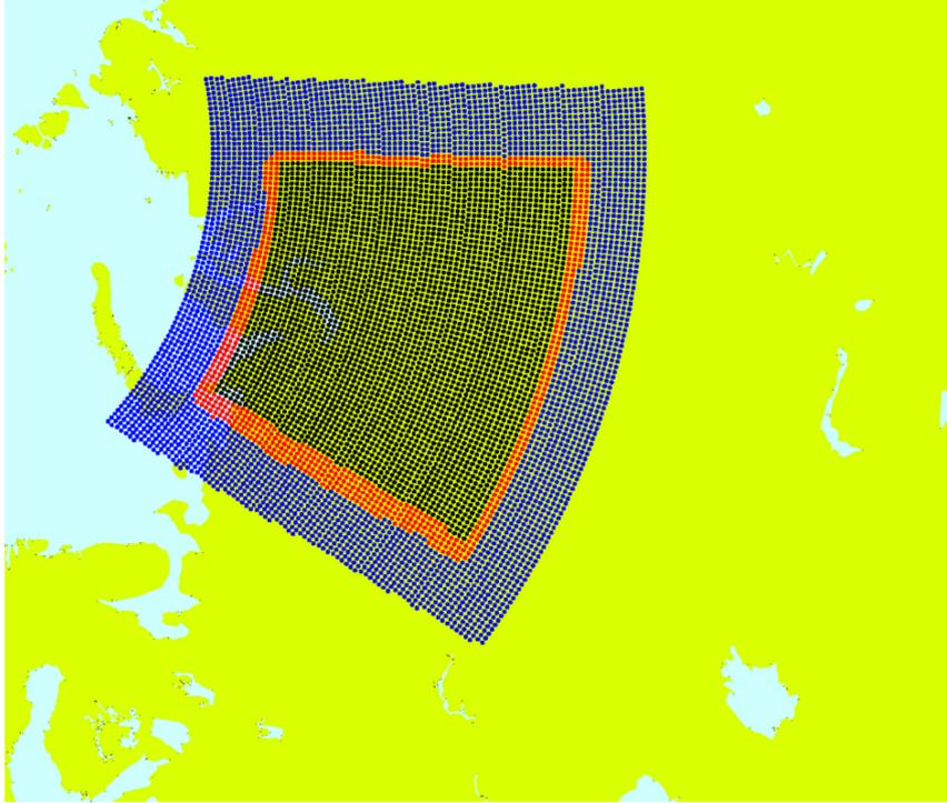
Figure 12: Original semi-Lagrangian transport, showing the halo grid-points that are actually used
