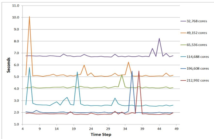
Figure 17: T3999L137 RAPS13 IFS (CY38R2) hydrostatic forecast model on TITAN (Cray XK7), cost per timestep
