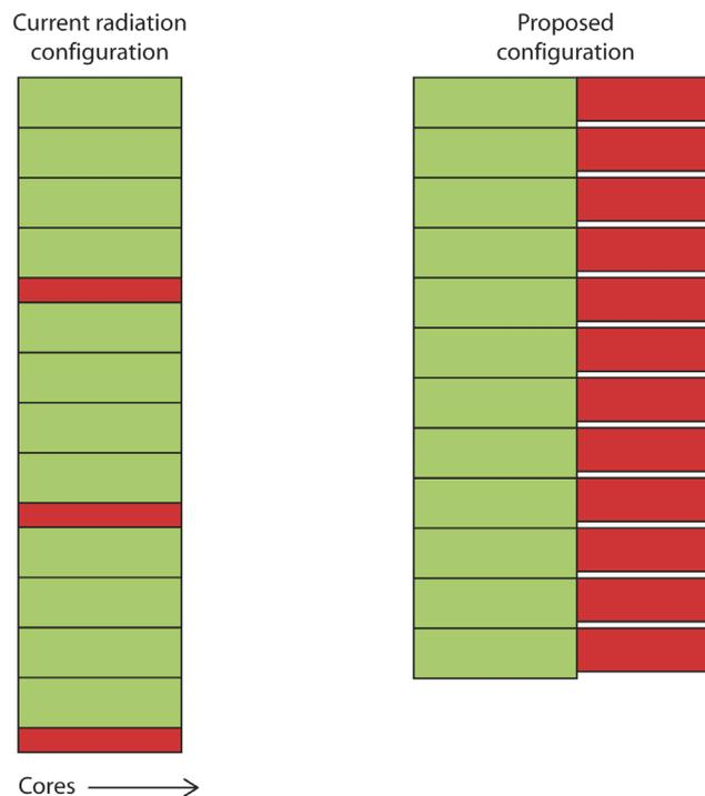
Figure 18: Schematic showing current and proposed radiation configurations. In the current configuration, non-radiation model timesteps are shown in green, and radiation computations are shown in red.
