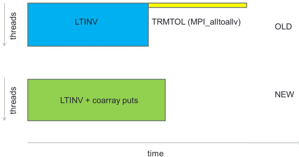
Figure 5: Schematic showing the overlap of LTINV computations with the associated TRMTOL transposition. (blue + yellow = green)
