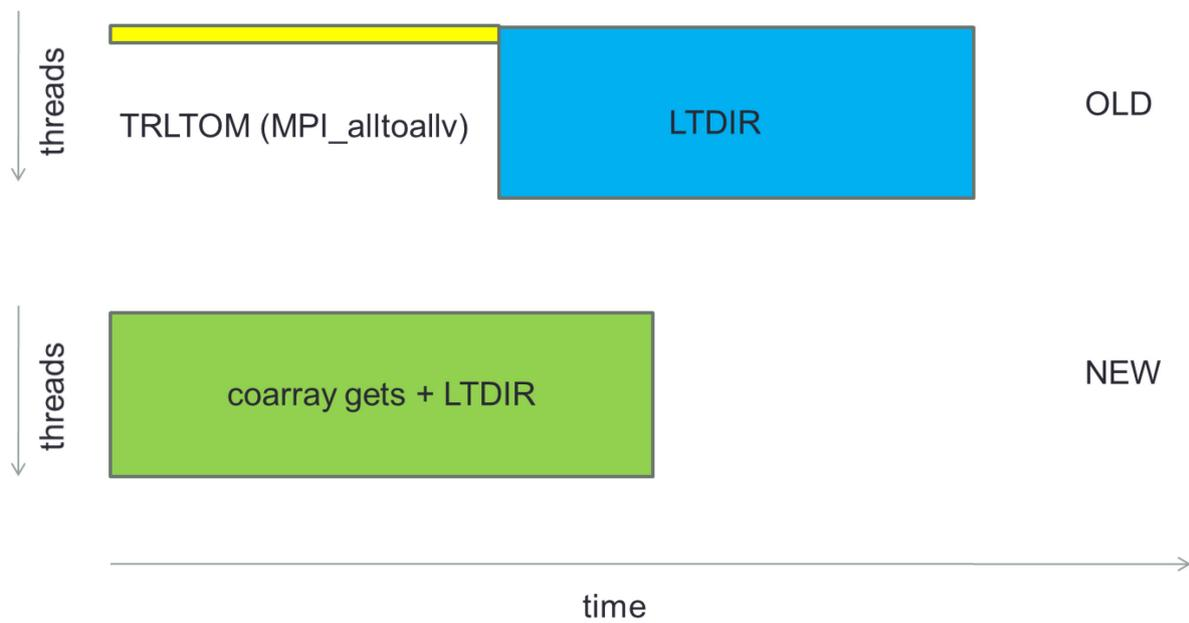
Figure 7: Schematic showing the overlap of LTDIR computations with the associated TRLTOM transposition
