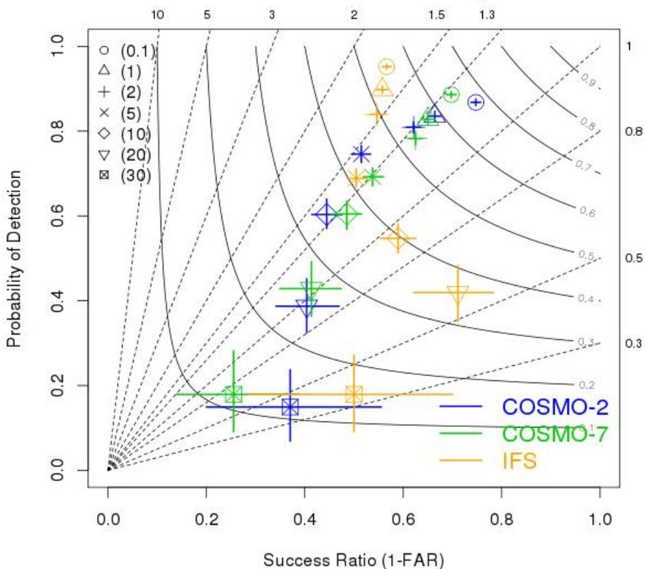
are compared to associated observations. For precipitation as one of the most important parameters, an example of a verification summary is shown in Fig. 2. Compared to COSMO-2 and COSMO-7, IFS shows a stronger overestimation of low precipitation amounts and also a stronger underestimation of high amounts. For thresholds of 5 mm/12 hours the values of all three models are quite similar.
