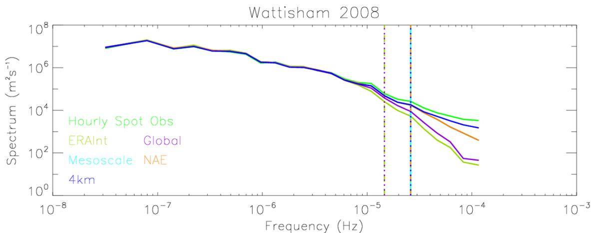
Fig. 3: Energy spectrum extracted from various NWP model configurations and observations for Wattisham over the entire year 2008.
