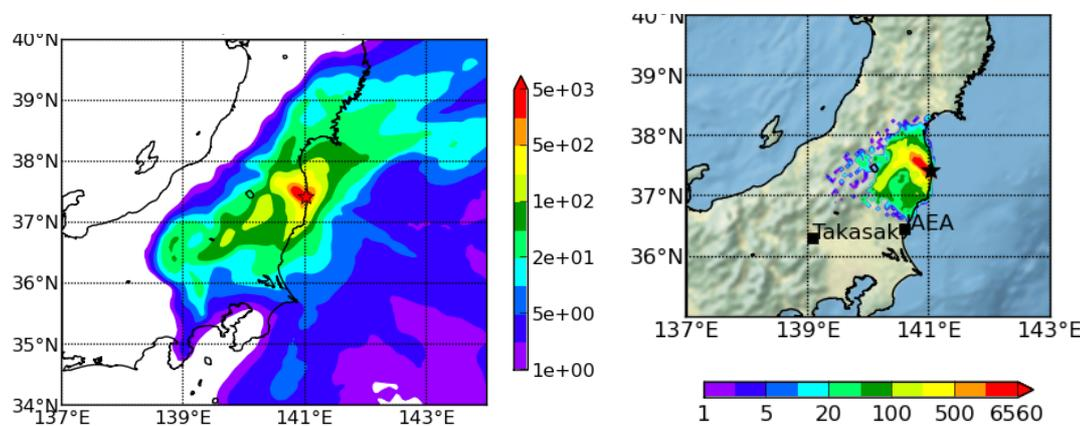
Fig. 2: Total (wet and dry) deposition of <sup>137</sup>Cs (in kBq/m<sup>2</sup>) during March 2011 predicted using NAME model runs with ECMWF meteorological data (left) compared to observed deposits (right)
