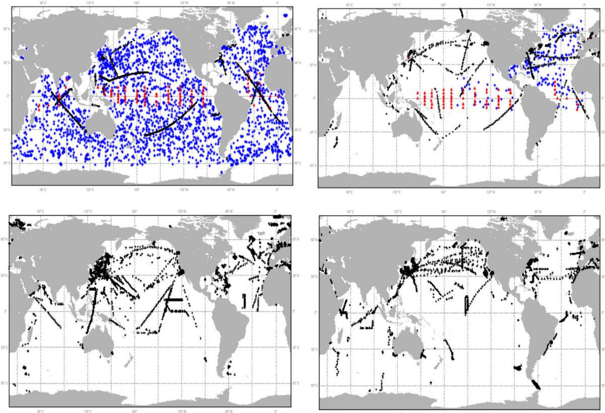
**Figure 3: Coverage at 10 year intervals from 1979 (bottom right), 1989, 1999 and 2009 (top left) for 10 day intervals. Note the vast improvement in coverage of the equatorial Pacific when the TAO array was developed (red dots), and the improved mid-latitude coverage when the ARGO system was developed (blue dots). Ten days is a typical data window used in ocean analysis systems.**
