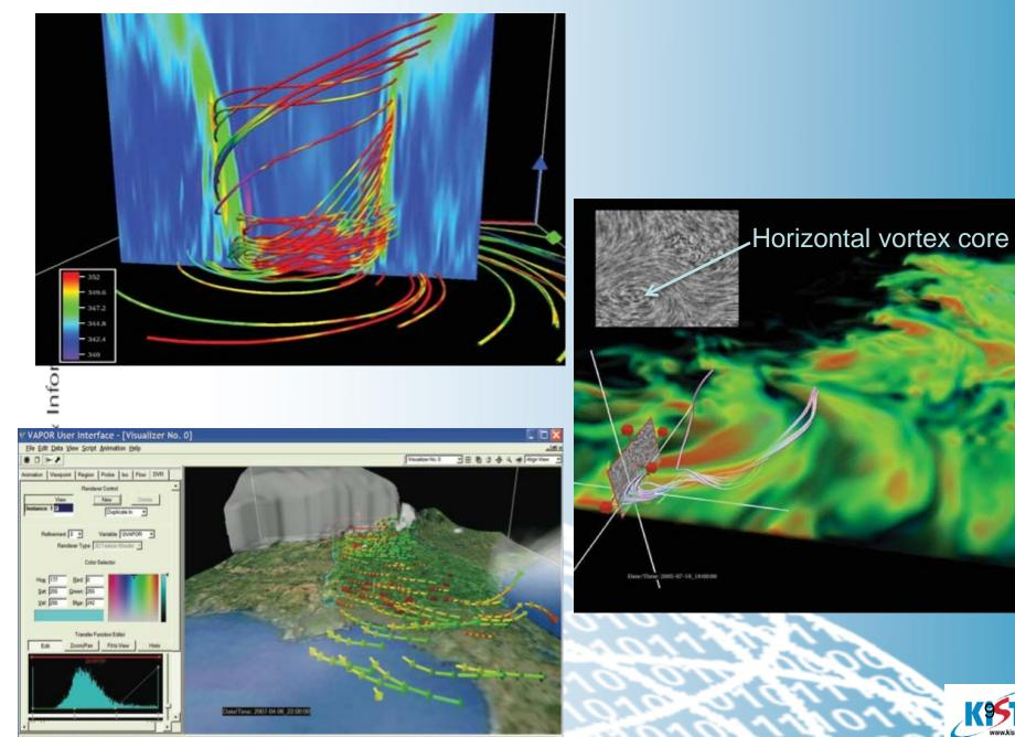
Rake Mode: To modify rake in scene, grab handle with left mouse to translate, right mouse to stretch
