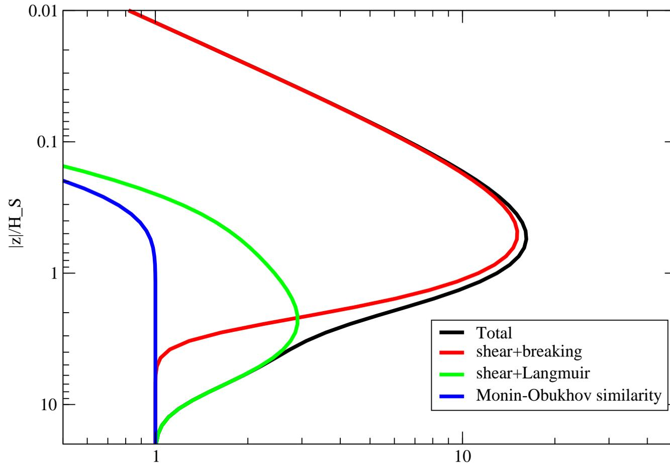
Figure 1: Profile of  $w = Q^3$  according to the local approximation in the ocean column near the surface. The contributions by wave dissipation (red line) and Langmuir turbulence (green line) are shown as well. Finally, the  $w$ -profile according to Monin-Obukhov similarity, which is basically the balance between shear production and dissipation, is shown as the blue line.
