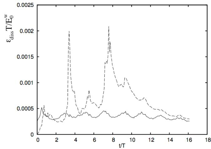
Figure 5: Dissipation nondimensionalized with period  $T$  and total energy in the water,  $E_0^w$  at  $t = 0$  as a function of nondimensional time for water (solid line) and air (dashed line). The initial steepness is 0.12
