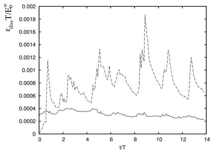
Figure 6: Dissipation nondimensionalized with period  $T$  and total energy in the water,  $E_0^w$  at  $t = 0$  as a function of nondimensional time for water (solid line) and air (dashed line). The initial steepness is 0.18
