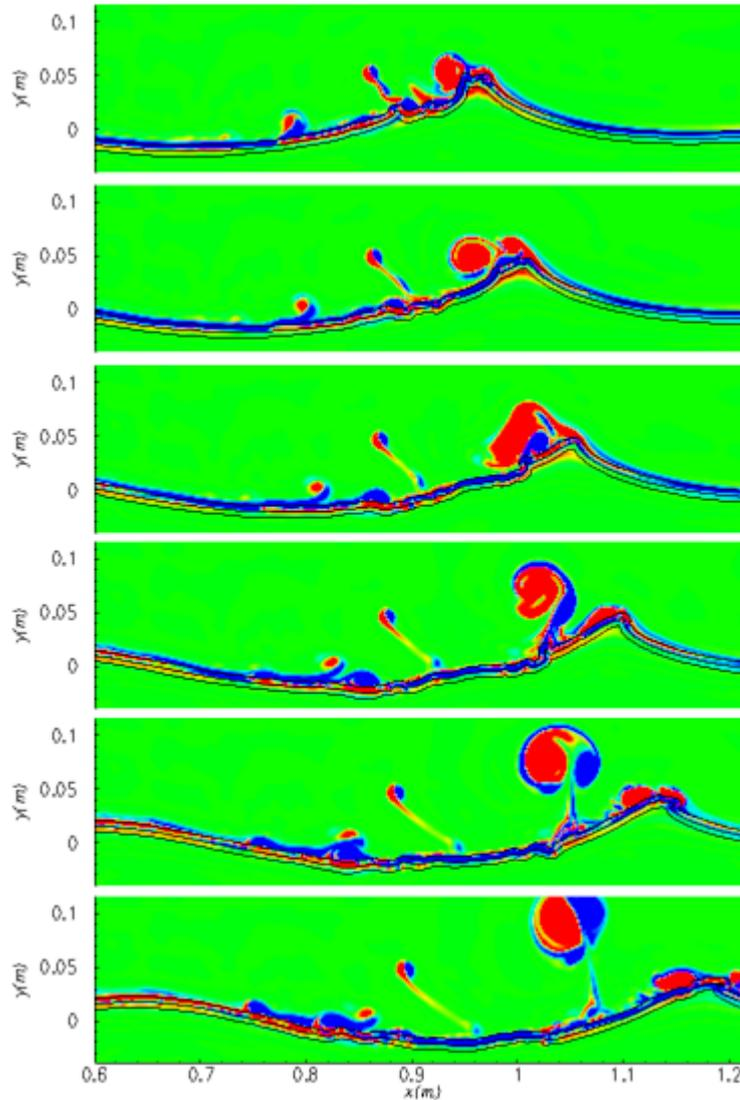
Figure 3: Sequence of formation of a dipole in air as a consequence of the wave breaking. The  $\Delta t$  between each image is 0.05 sec. The initial steepness is 0.18
