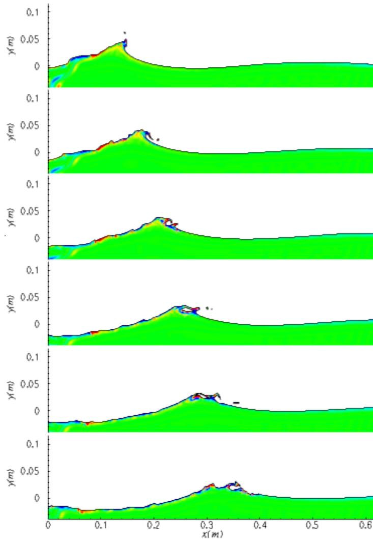
Figure 2: Breaking event for initial steepness  $\epsilon_0=0.18$ . The color corresponds to the vorticity field: green corresponds to zero vorticity, blue to  $-20 \text{ sec}^{-1}$  and red to  $20 \text{ sec}^{-1}$ . The  $\Delta t$  between each image is 0.05 sec.
