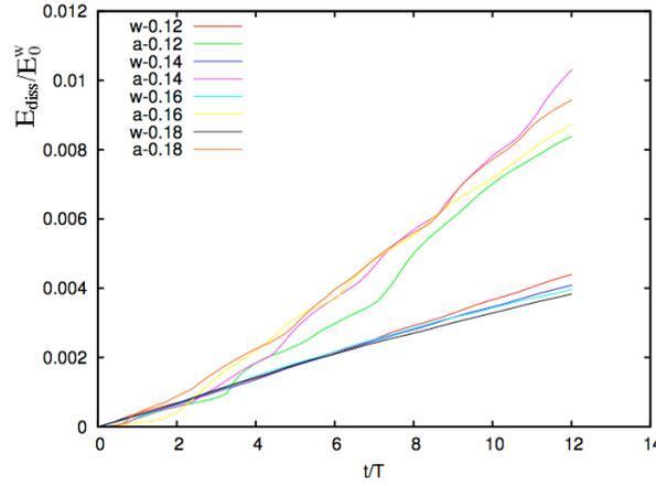
Figure 7: Integrated dissipation for different values of the steepness in water (w) and air (a).
