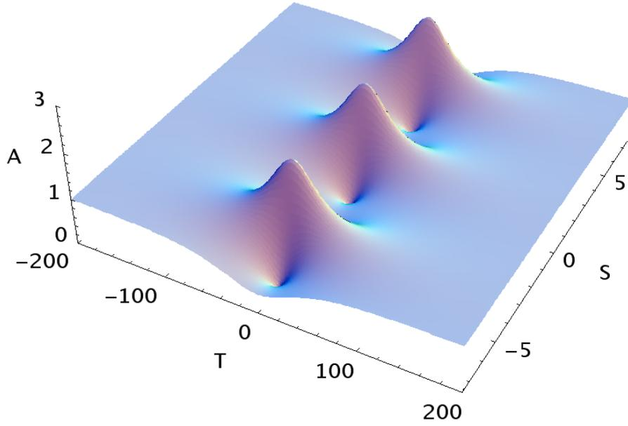
Figure 1: The Akhmediev solution: normalized wave envelope as a function of nondimensional time and space
