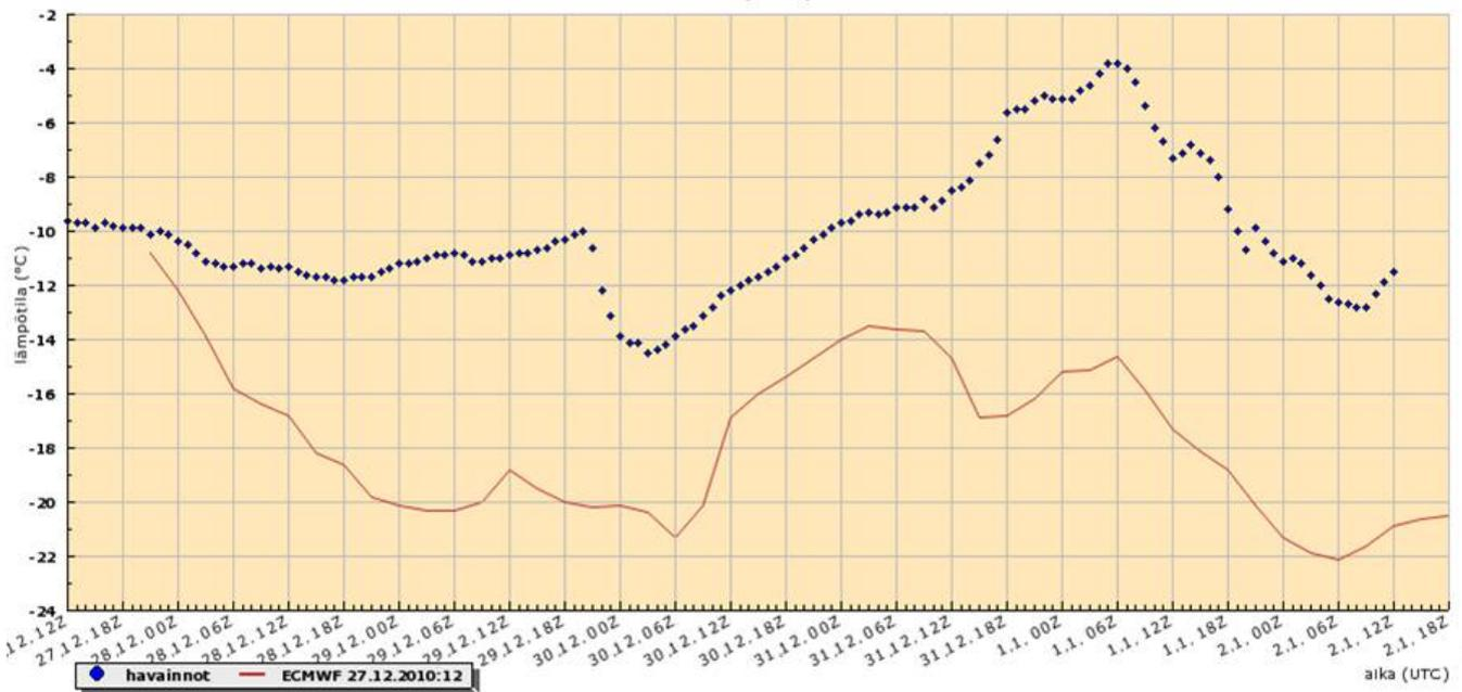
**Figure 5** ECMWF forecasts and observations at the turn of the year 2010–2011 in Tampere (27.12.2010 – 2.1.2011). The red curve shows the forecasted temperature and the blue dots show the observations.
