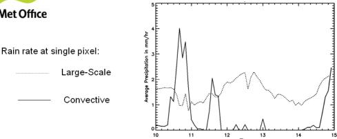
Radar rainfall rates used hourly from T-2 to T+3 Equivalent background values are averaged over 30 minutes
