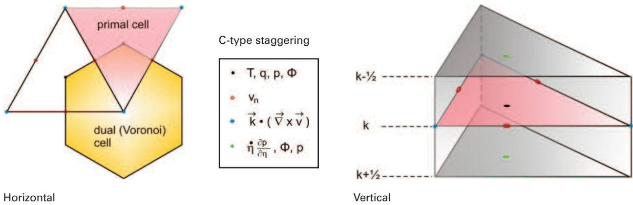
**Fig. 6** 3D arrangement of discrete variables
