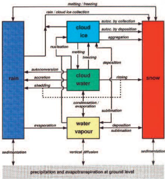
**Fig. 3** Processes of the cloud microphysics scheme of GME30L60 (grid scale)
