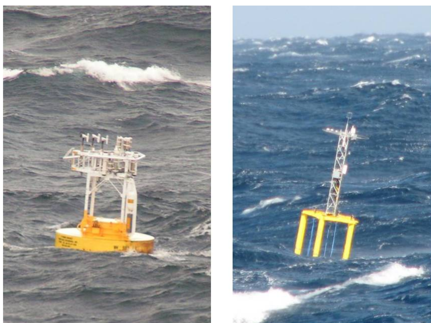
Figure 3. Two of the platforms used during the CLIMODE program to provide direct covariance estimates of the momentum and heat fluxes. The 3-m discus mooring that was successfully deployed for 15 months in the Gulf Stream is shown at left, while the Air-Sea Interaction Spar (ASIS) is shown at right.
