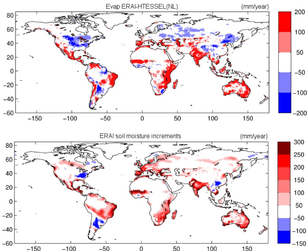
Figure 7: Top panel: yearly evapotranspiration difference between ERA-Interim and HTESSEL (NL) simulation. Bottom panel: annual mean soil moisture increments (top three layers) from the assimilation during ERA-Interim reanalysis.
