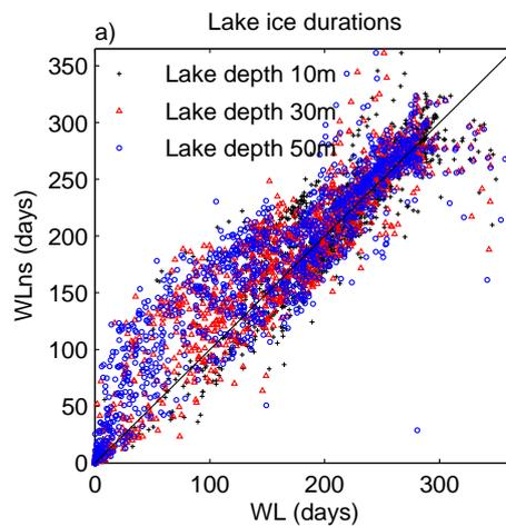
Figure 8: Mean lake ice duration simulations from WLns (with lake, no snow with lake ice albedo given by eq. 1) versus the same quantity for WL (with lake) simulations.
