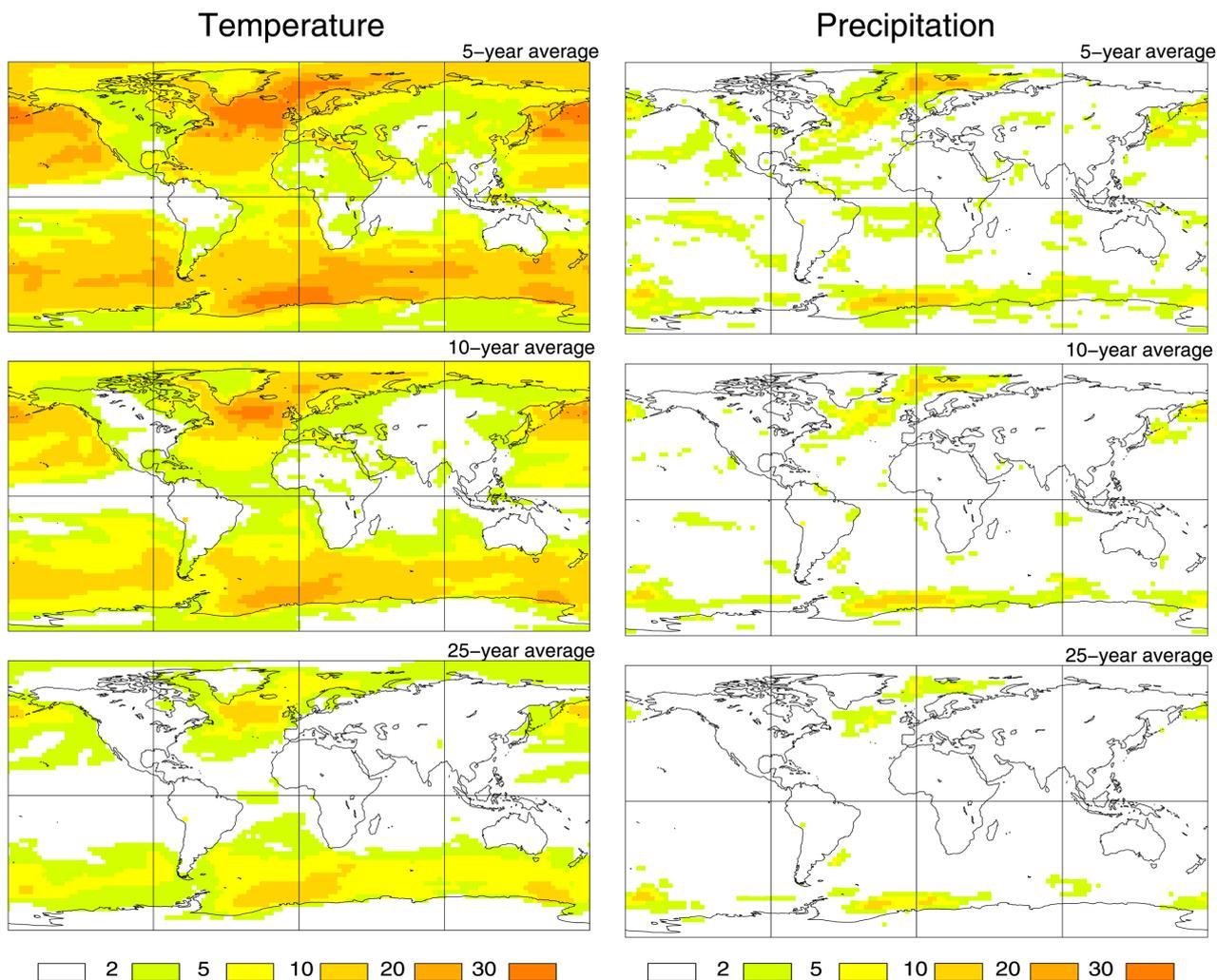
Figure 2: Estimated potential predictability variance fraction (ppvf) expressed as a percentage for 5, 10 and 25 year averages for temperature (left) and precipitation (right). Potential predictability of precipitation is much less than that for temperature though the patterns are similar. Over land potential predictability is small for both temperature and precipitation. From Boer and Lambert (2008).
