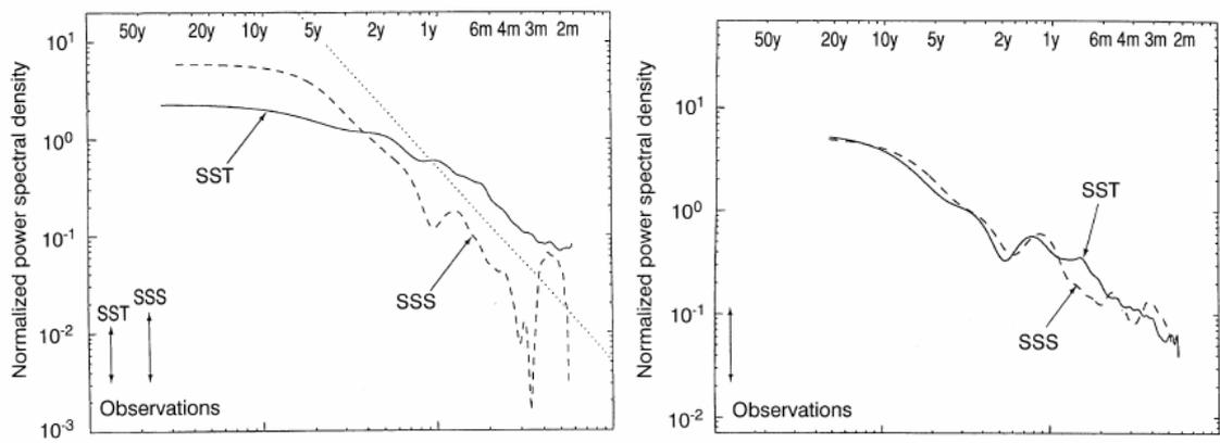
Figure 1: Spectra of sea surface temperature and sea surface salinity at ocean weather stations Papa (North Pacific) and India (North Atlantic). The spectra for Papa are consistent with local stochastic forcing by the atmosphere with the atmospheric spectrum being white. A different story applies in the North Atlantic, where the  $T$  and  $S$  spectra are very similar. From Hall and Manabe (1997).
