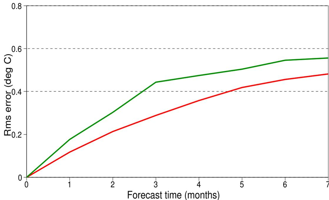
Figure 16: Plot of the rms error in the Niño 3.4 region as a function of forecast lead time for two sets of hindcasts. Green corresponds to the forecasts initialised using just SST, while red corresponds to hindcasts from initial conditions using all available oceanic and atmospheric data. The skill of the forecasts initialised just using SST data is significantly worse than the skill of those initialised using oceanic and atmospheric observations. From Balmaseda and Anderson (2009).
