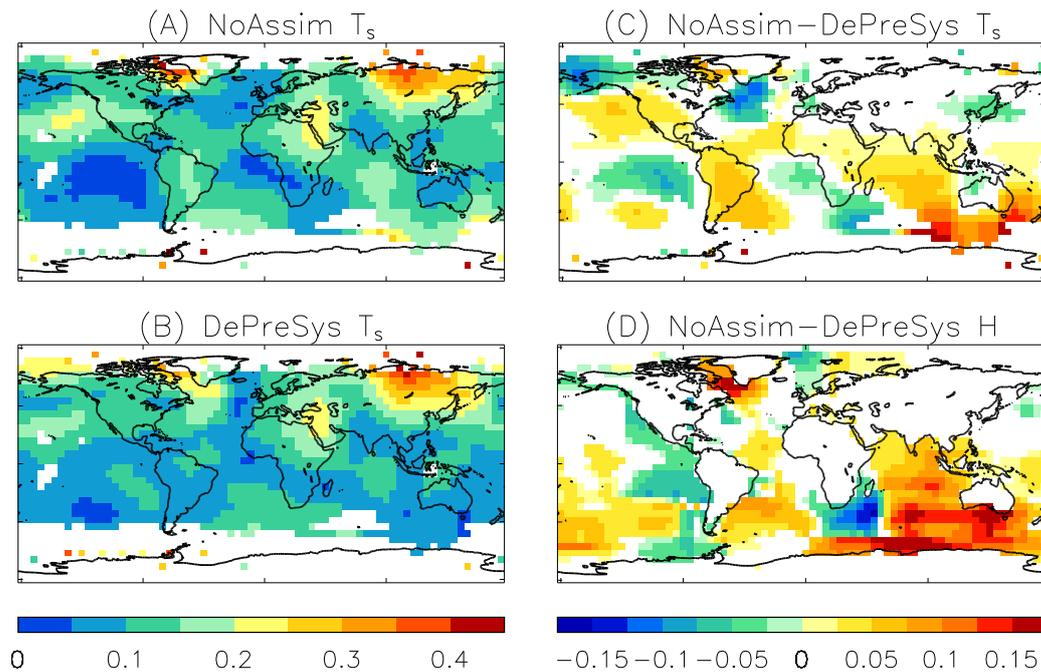
Figure 12: Impact of initial conditions on forecast skill. A and B indicate rms error of 9-year mean hindcasts of near-surface temperatures for the uninitialised and DePreSys hindcasts initialised over the period 1979-2001, and C shows the differences where they are significant. D is similar to C but for upper ocean heat content. From Smith et al. (2007).
