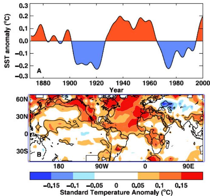
Figure 4: Upper) Plot of the low frequency variability in the North Atlantic SST represented by the AMO index. Lower) Surface temperature anomaly associated with one positive standard deviation of the AMO. Based on observations, from Knight et al. (2005).
