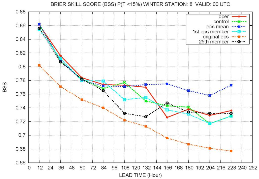
Fig. 2 Wintertime Brier Skill Score (BSS) of ECMWF EPS temperature forecasts corrected with Kalman filtered operational, control, EPS mean, 1<sup>st</sup> individual EPS member, 25<sup>th</sup> individual EPS member and original EPS, averaged over eight stations in Finland.
