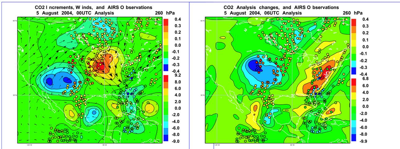
Figure 6: CO<sub>2</sub> increments at 21 UTC (left) and CO<sub>2</sub> analysis changes at 6 UTC (right) at model level 32 for two AIRS overpasses between 7 UTC and 8 UTC (shown as dots using the observation departure value for the color scale). Wind vectors for the same model level are overlaid in the left panel to illustrate the main horizontal advection pattern.
