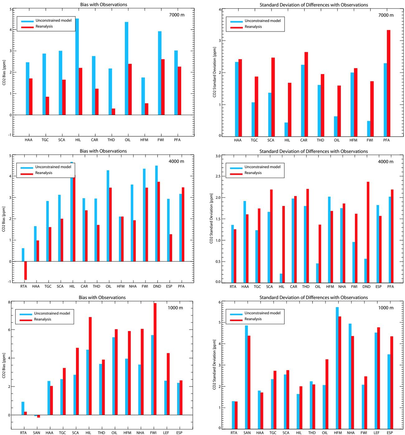
Figure 4: Bias (left) and standard deviation of the difference (right) of the unconstrained model run (blue) and the AIRS reanalysis (red) relative to independent flight observations from the NOAA/ESRL network
