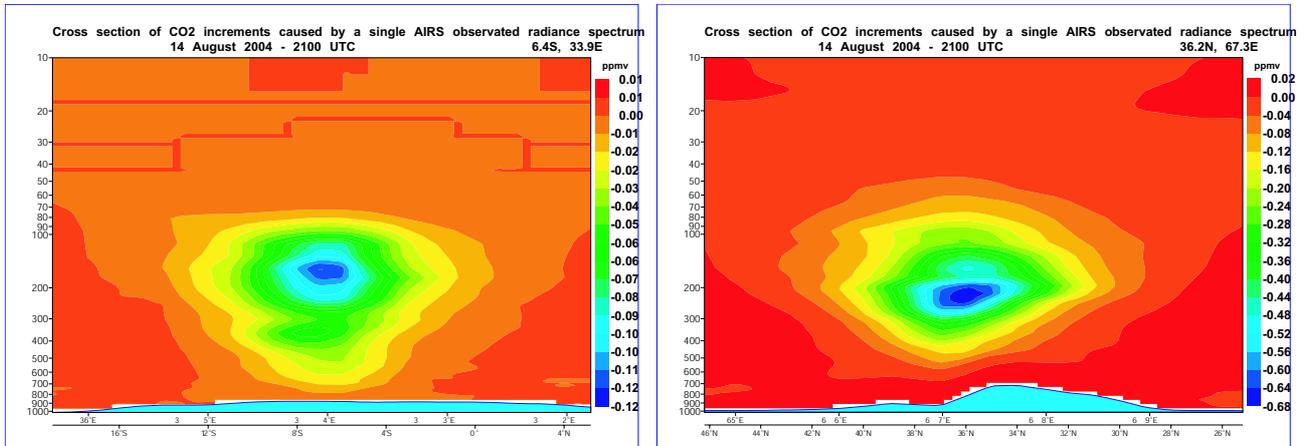
Figure 3: Vertical cross sections of CO<sub>2</sub> increments caused by a single AIRS observation (using 24 CO<sub>2</sub> sensitive channels) over tropical Africa (6.4°S, 33.9°E) and over mid-latitude Asia (36.2°N, 67.3°E).
