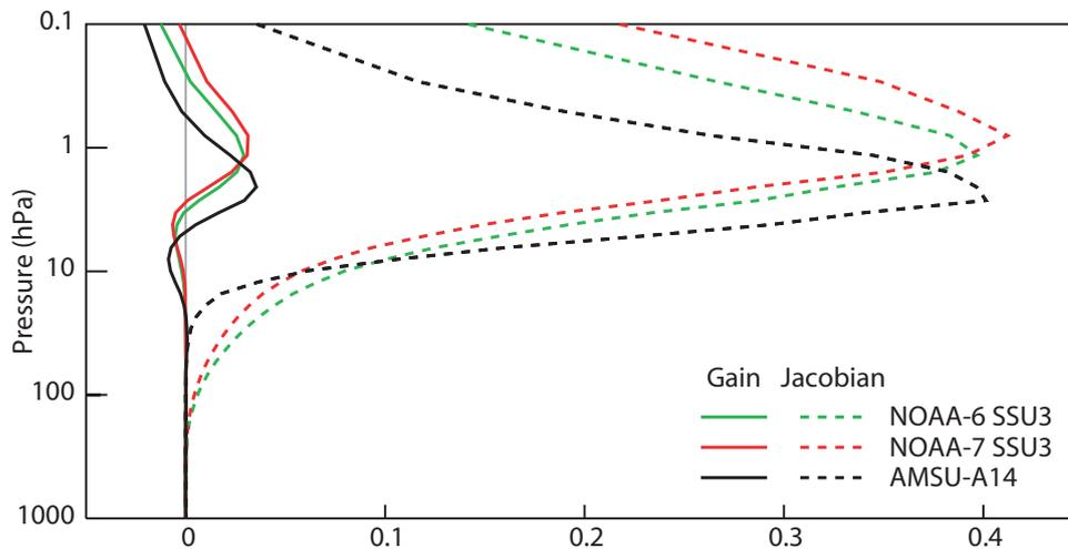
Figure 17: Jacobians and gain vectors for the highest-peaking channels of SSU and AMSU-A, from Kobayashi *et al.* 2008.
