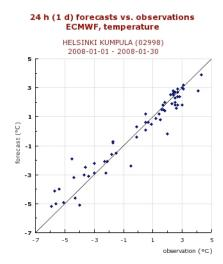
Fig. 6 Example of scatter plot of forecasts vs. observations of the new verification system.
