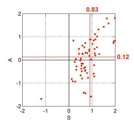
Fig. 14 Scatterplot of the S (structure) and A (amplitude) components of the SAL verification measure for ECMWF 30-hour deterministic QPFs for Kokemäenjoki river catchment during winter 2007-2008. There are 63 analysed cases and each S/A combination is represented by a solid blob. The dotted lines represent the mean values of S and A, averaged over the dataset.
