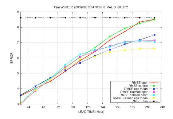
Fig. 1 Wintertime RMS Error of operational, control and EPS mean temperature forecasts and corresponding Kalman filtered forecasts, averaged over eight stations in Finland.
