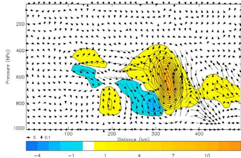
Evaporative cooling leads to enhanced descent beneath the frontal cloud band **and** enhanced ascent in the frontal updraught
