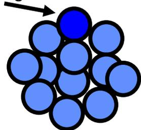
Curved surface: saturation vapour pressure increases with smaller drop size since surface molecules have fewer binding neighbours.
