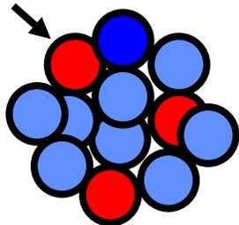
Presence of dissolved substance: saturation vapour pressure reduces with smaller drop size due to solute molecules replacing solvent on drop surface (assuming  $e_{\text{solute}} < e_v$ )
