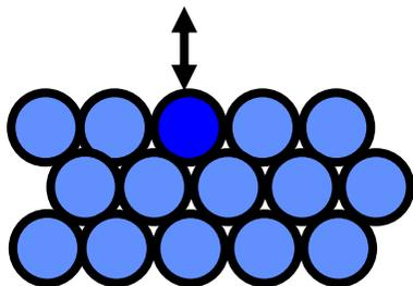
Planar surface: Equilibrium when  $e=e_s$  and number of molecules impinging on surface equals rate of evaporation
